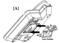
**[A]:** For the Holder fixed, you can follow the picture to do it. First, you need to fixed the Low Holder, the steps is from "a" to "b".
