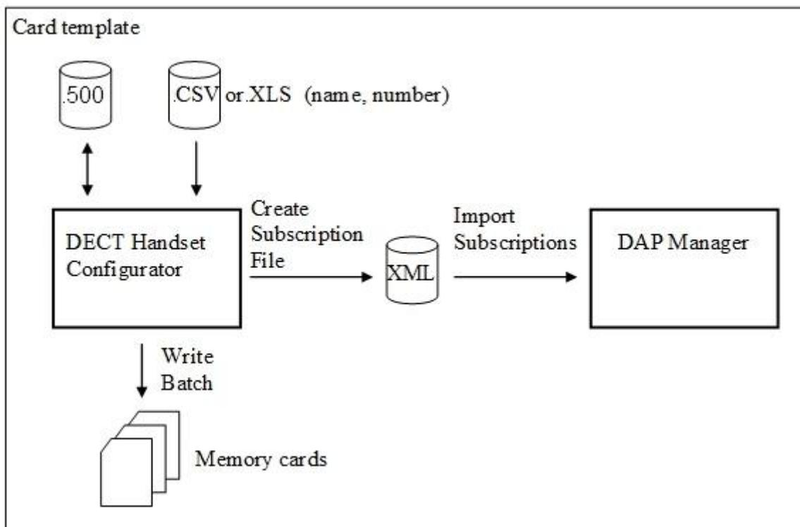
1. Using the DECT Handset Configurator a [Subscription File](#) (.XML) is created (Tools->Create Subscription File). Input is a [CSV File](#) containing the names and numbers of all handset users. Alternatively a [Central Directory Database](#) (file type .XLS) may be used. The user also enters the PARI of the DECT system and selects the directory where the output XML Subscription File will be stored.
