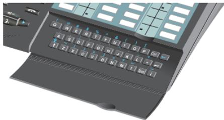
The keypad is used for mail service functions, the "Call by name" function and for programming.
