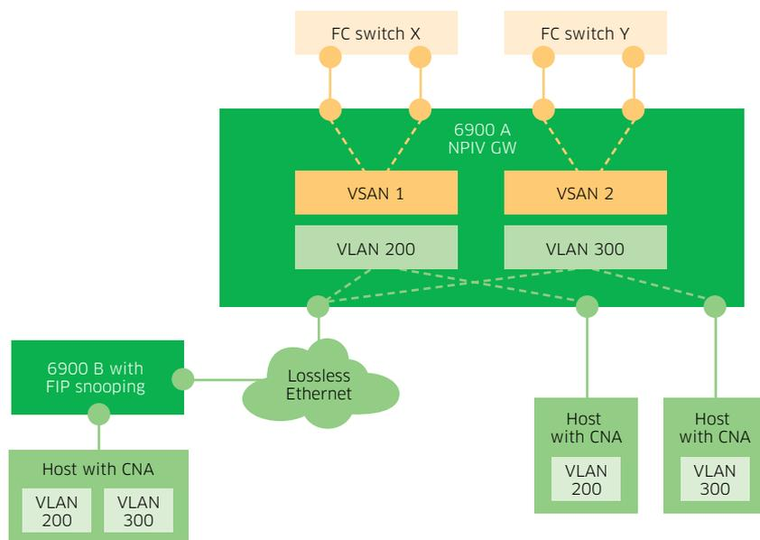
Figure 1 shows a standalone switch operating as a NPIV gateway connecting the Ethernet and FC networks. VSAN 1 is mapped to VLAN 200, and VSAN 2 is mapped to VLAN 300. The switch acts a proxy for all the Ethernet devices to the fiber channel switch. The switch can support up to one SAN per interface
