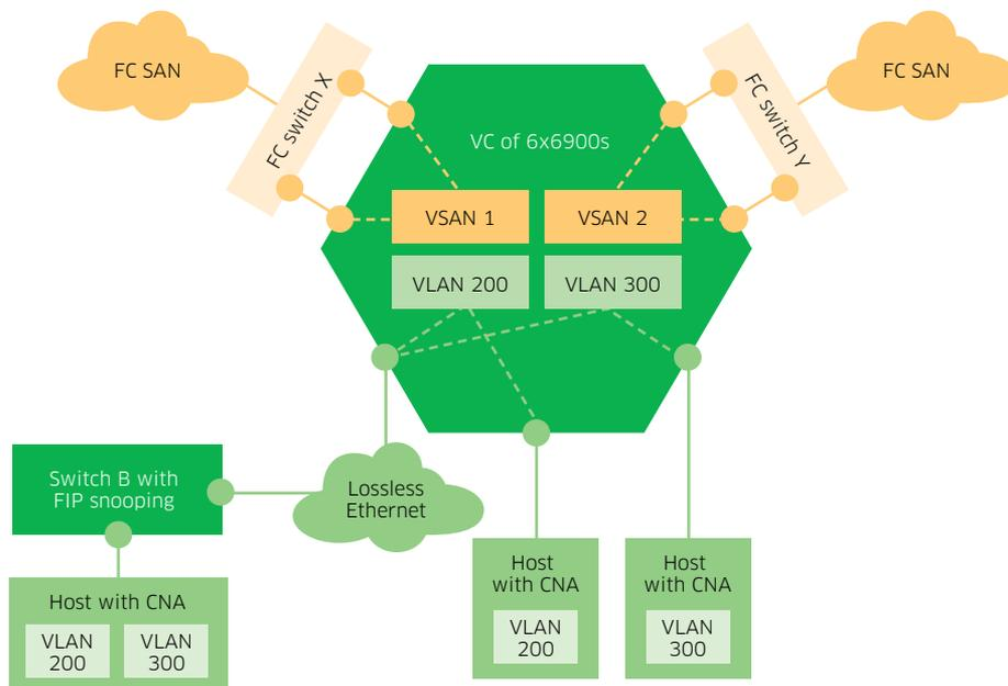
An Alcatel-Lucent OmniSwitch™ 6900 with an FC interface performing the tunnel operation would be termed an initiator; the remote endpoint (either FCF or E\_port tunnel) is referred to as a target.
