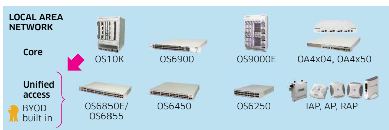
Figure 9. The simplified, flatter architecture of the Alcatel-Lucent Enterprise Converged Campus Network Solution
